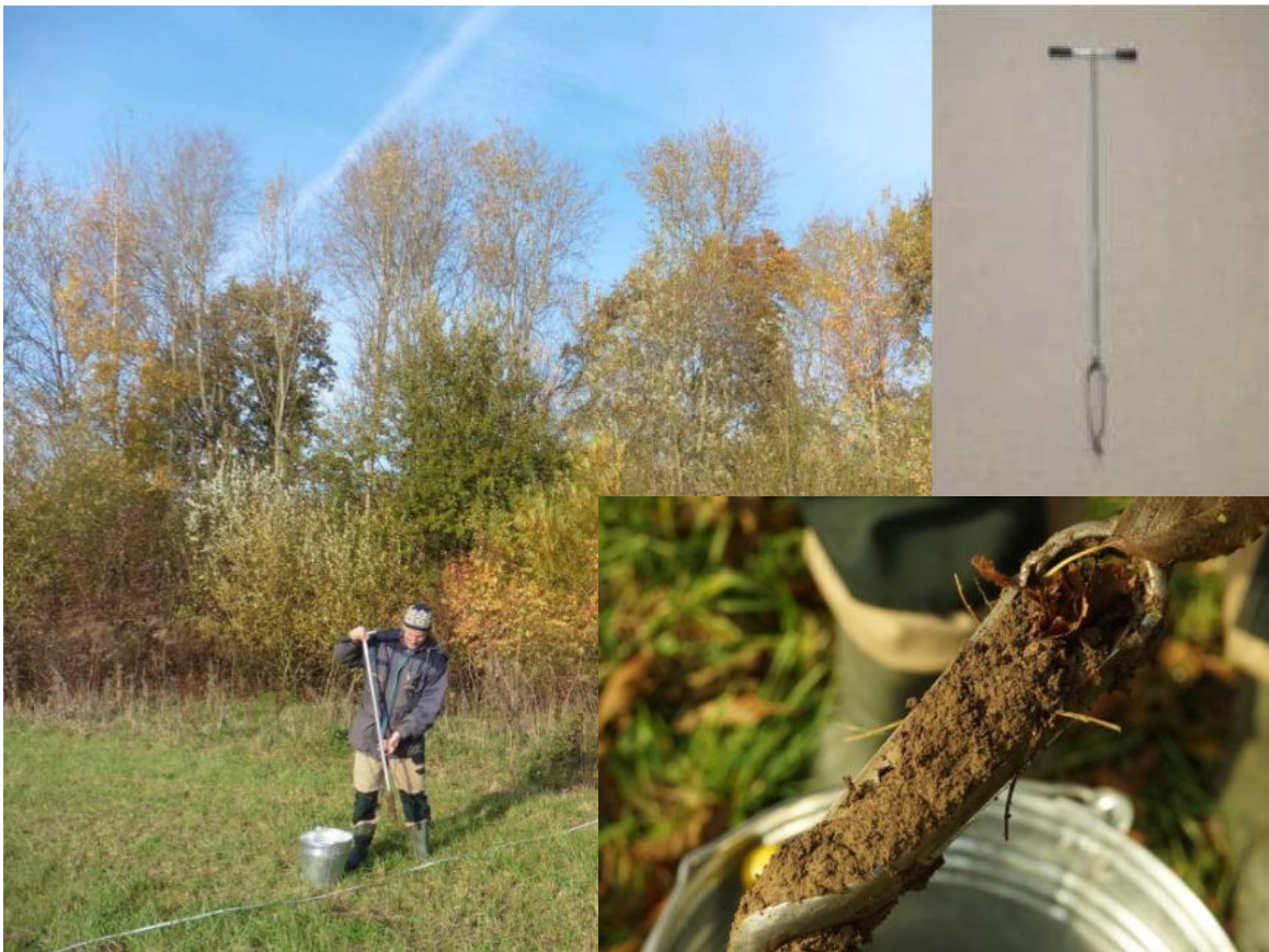
Figure 2. Sampling auger used to take soil samples
